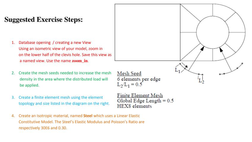
5. Create a 3-D element property named, Solid\_Elements\_Steel, for the entire includes the steel material definition
