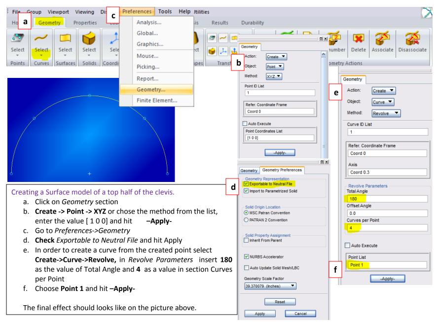
You will now use Curvilinear transformation to create the outer radius of the lug by radially translating the curves that define a quarter of the hole.
